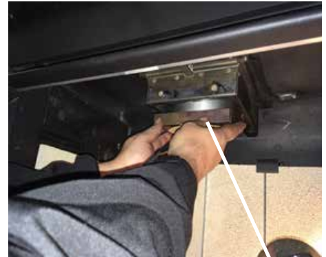
Install square support and catalyst into cartridge
