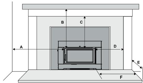
**Minimum Hearth Extension for the front (E) and sides (F) are measured from the fuel door opening.**
