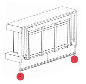
**18)** Install the bottom panel onto the underside to the surround with the four surround screws left over.
