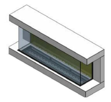
For a two-sided (cornered) Firebox screws installation, add one of the blanking plates and secure with the six firebox screws into position. Next add the two small trims and the large trim to the side of the appliance. Then line the holes of the trims with the corresponding holes of the firebox and screw into position with the six countersunk screws, previously removed.
