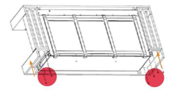
17] Underneath the appliance, with the surround screws, screw up through the bottom surround and into the legs of the surround top section and up through the floating shelf brackets on the appliance the top section.
