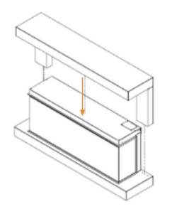
**16**) Carefully lower the top section of the surround onto the top of the firebox.
