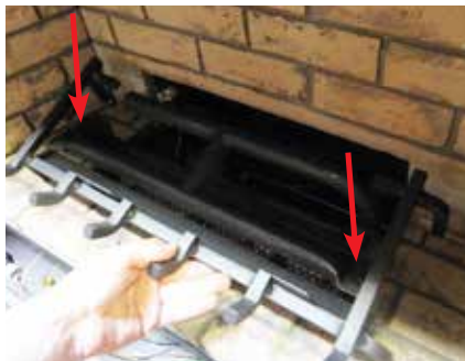
Diagram 1: Remove the left and right screws.
