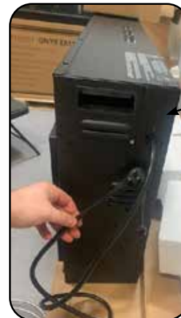
Wire Harness & Cover Plate Reinstalled.
