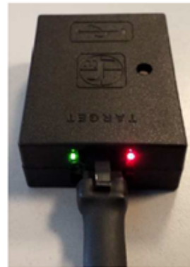
Fig.3: WiFi dongle connected to the IFC
